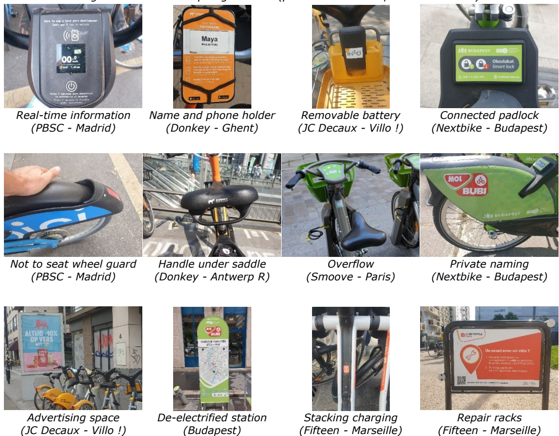
Figure 18: Several inspiring features (photos: B. Beroud | Overflow: SAVM)
